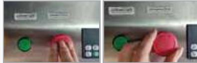
In case of emergency, you can press the red stop button, lock the equipment, need to spin, turn and bounce and open the button, before the next operation can be performed normally.
